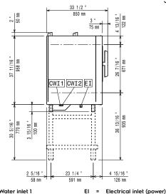
CWII Cold Water inlet 1 CWI2 Cold Water Inlet 2
